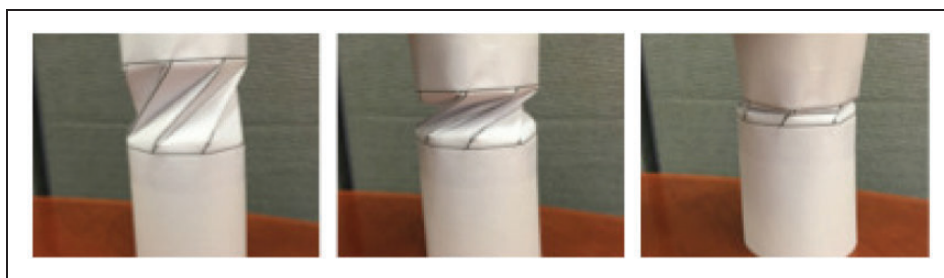
Figure 10. Foldable cylinder based on twist buckling.
